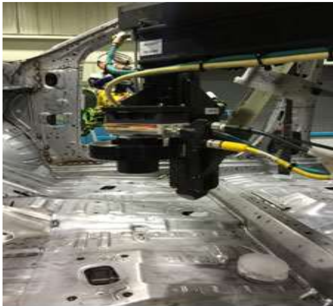
A 2D vision guided robot performs bolt shooting and tightening on automotive underbody. (Courtesy of Recognition Robotics Inc.)
