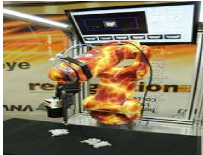
Robot picks and stacks randomly piled parts in six degrees of freedom without calibration, CAD files, lasers or point clouds. (Courtesy of Recognition Robotics Inc.)
